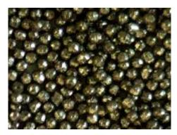
**Typical Applications:** Shot peening, including but not limited to airframe parts, turbine parts, aerospace and automotive engine and gear components, springs, and suspension parts.
